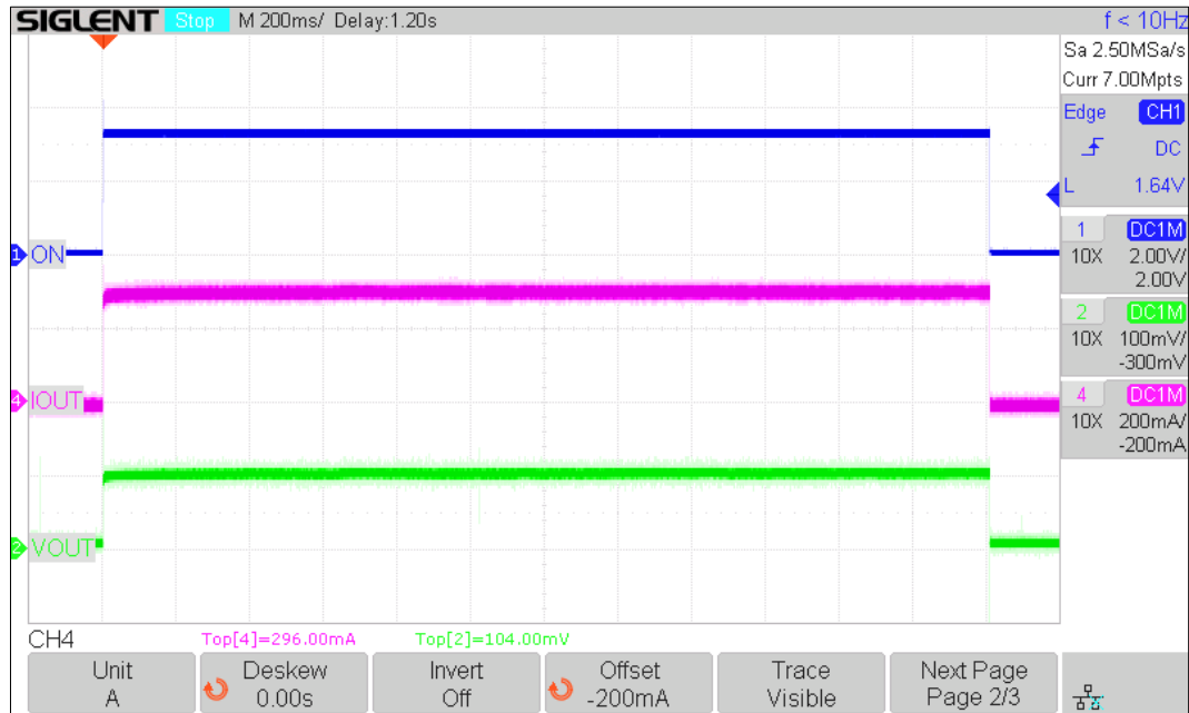
Figure 9. AM6U1404 SCL Operation Waveform. V_{DD} = V_{IN} = 3.3V , R_{LOAD} = 0.3\Omega , C_{OUT} = 10\mu F , C_{SLEW} = 3.9nF .
