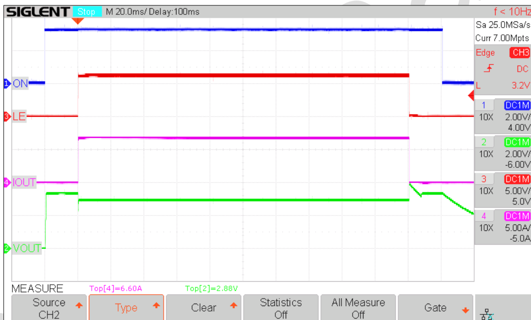
Figure 8. AM6U1404 ACL Operation Waveform. V_{DD} = V_{IN} = 3.3V , R_{LOAD} = 20\Omega , C_{OUT} = 10\mu F , C_{SLEW} = 3.9nF . Load Enable signal applies an additional 0.4\Omega of load.
